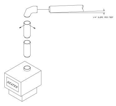
FIGURE 2.3 (B) Minimum Slope
